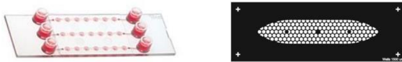
Figure 6. \mu -Slide Spheroid Perfusion from ibidi® (left) and PDMS LOC device (right).
